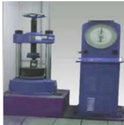
Fig.9 compressive strength testing machine
