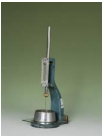
Fig.3 cement mortar setting time machine
