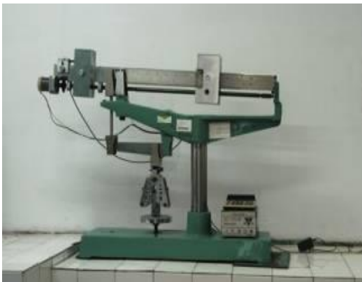
Fig.8 bending strength testing machine
