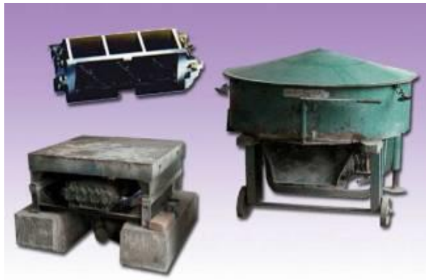
Fig.1 concrete mixer, vibrating table, die
